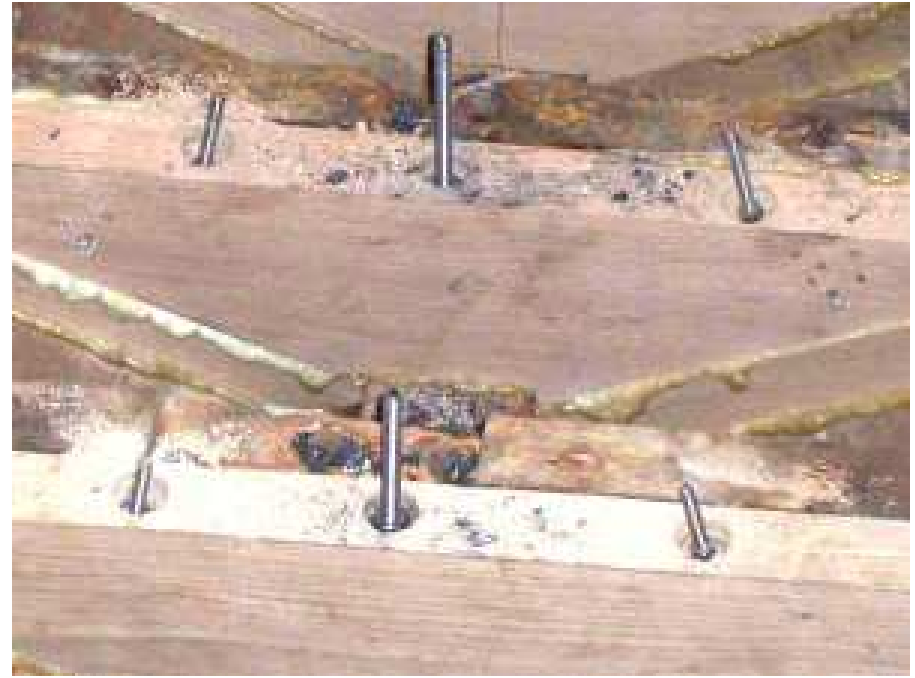
sample with three bolts, middle through the keel
