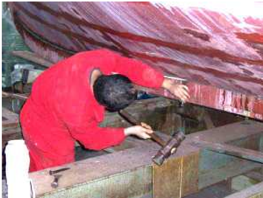
drive into cotton between keel and garboard
