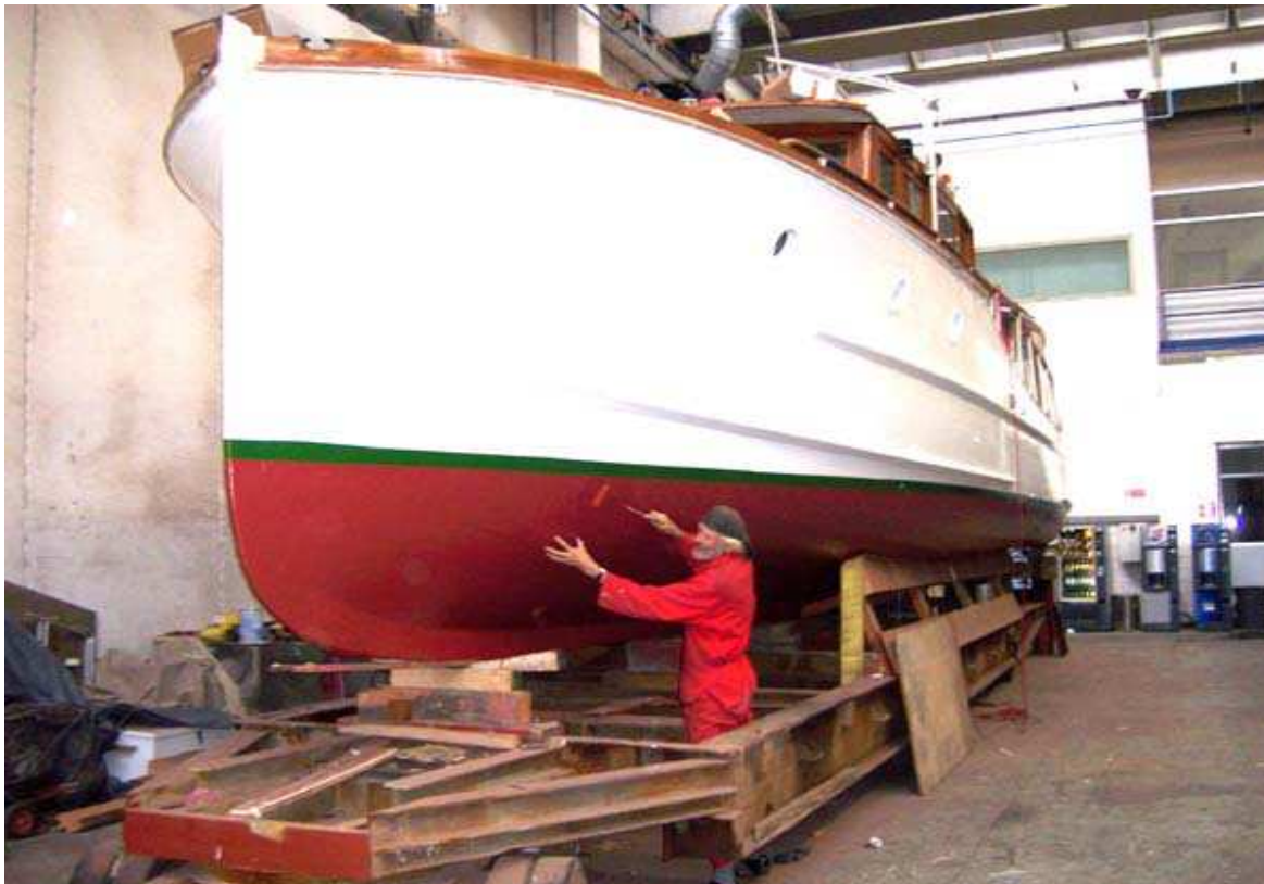
sealing with poleuretlan rubber
