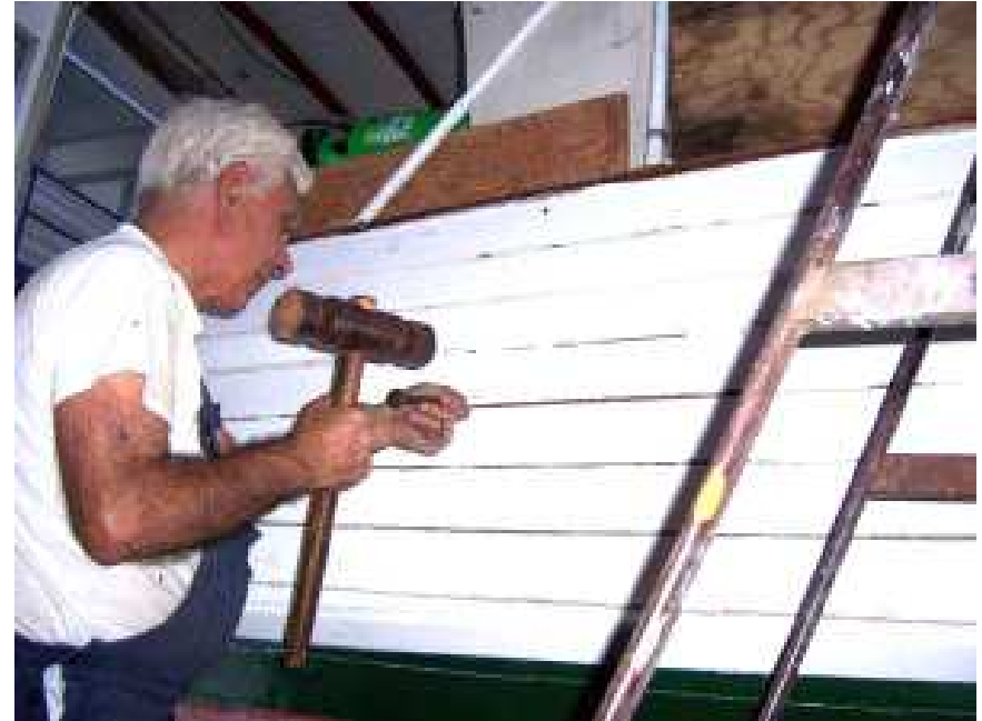
80 year old Stefano caulking
