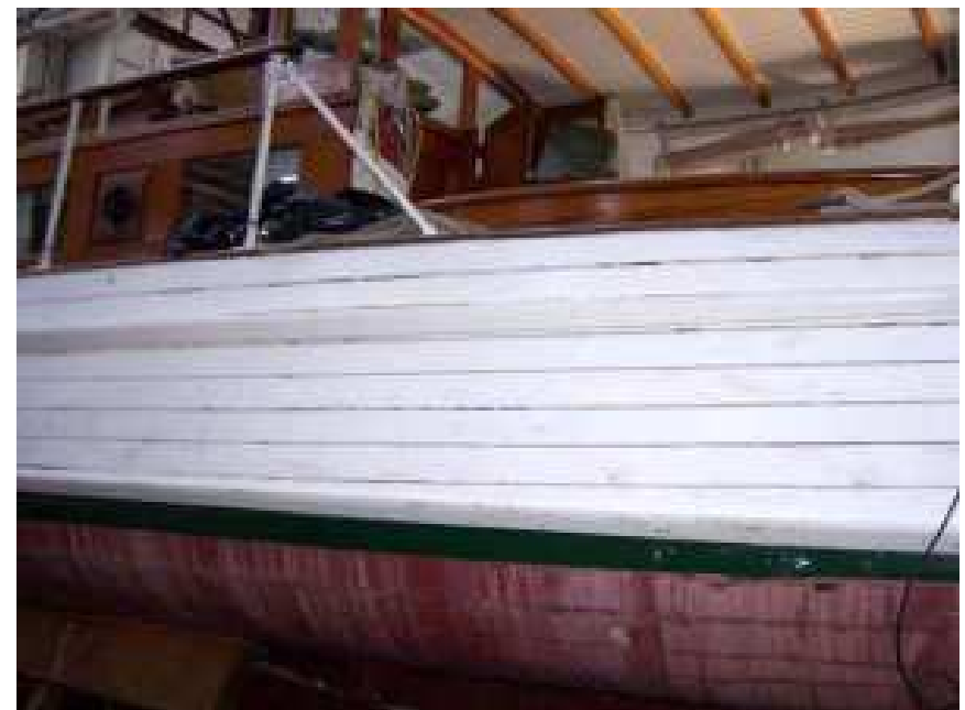
all breaks between planks caulked
