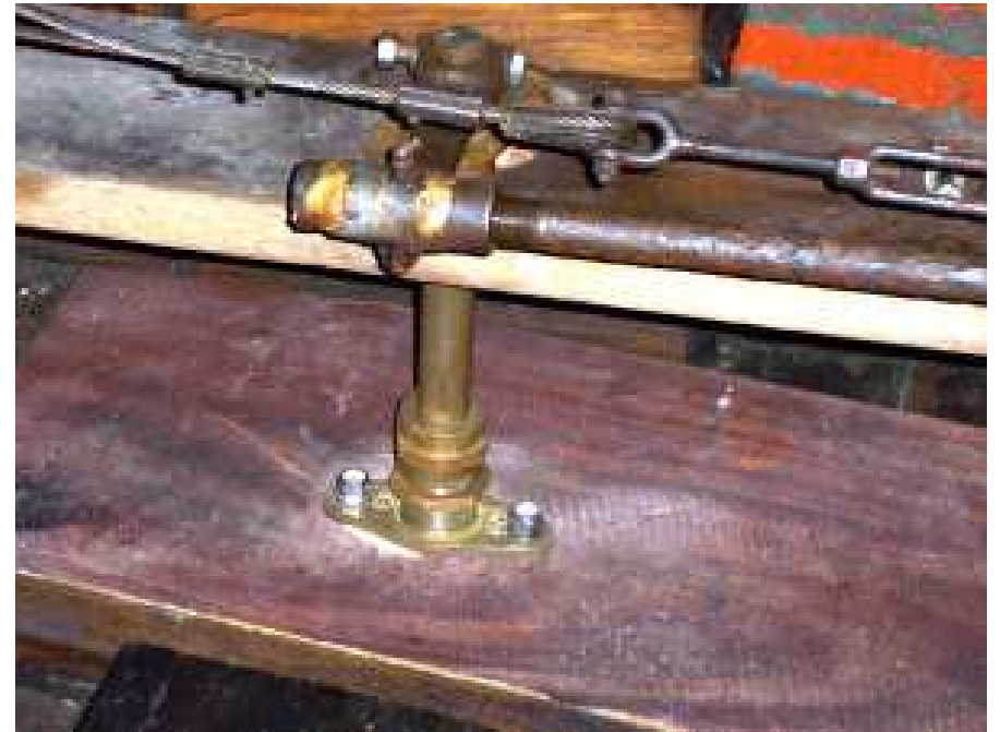
large new board under the rudder fittings
